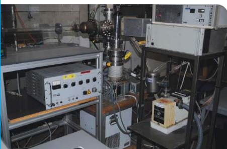
Mass spectrometer coupled to a DC glow discharge tube
