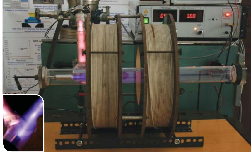
Helmholtz coil confining electrons in a discharge tube, 2 focal points on the discharge axis
